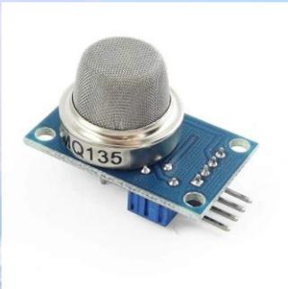
SENSOR MQ-135, SE HA USADO PARA MEDIR EL CO<sub>2</sub>
